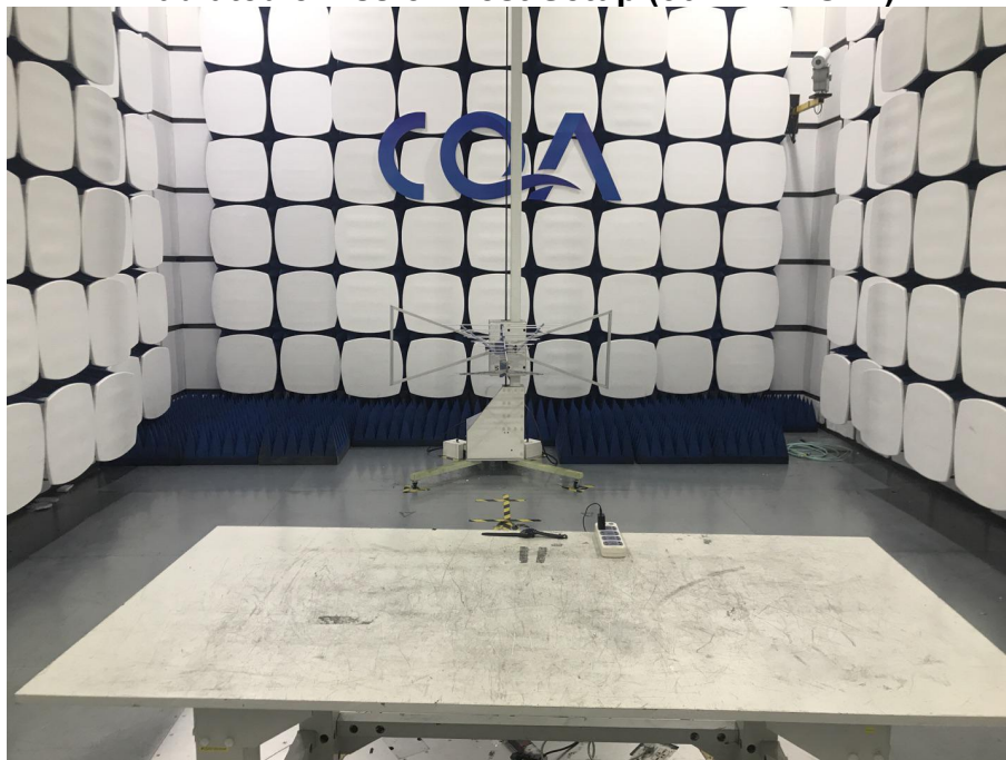
Radiated emission Test Setup (30MHz~1GHz)
