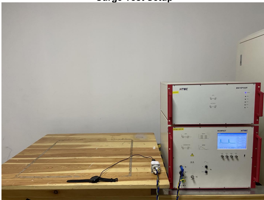
Surge Test Setup
