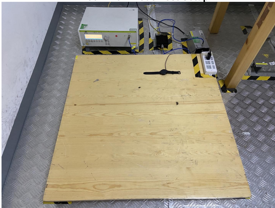
RF common mode Test Setup
